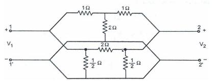
**b** Express Z-parameters in terms of h-parameters for a two port network.
